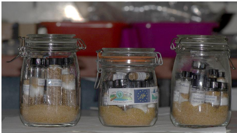
Figure 2: Leak-proof glass containers stored into larger leak-proof glass containers on top of silica gel (photo from S. Oikonomidis).
